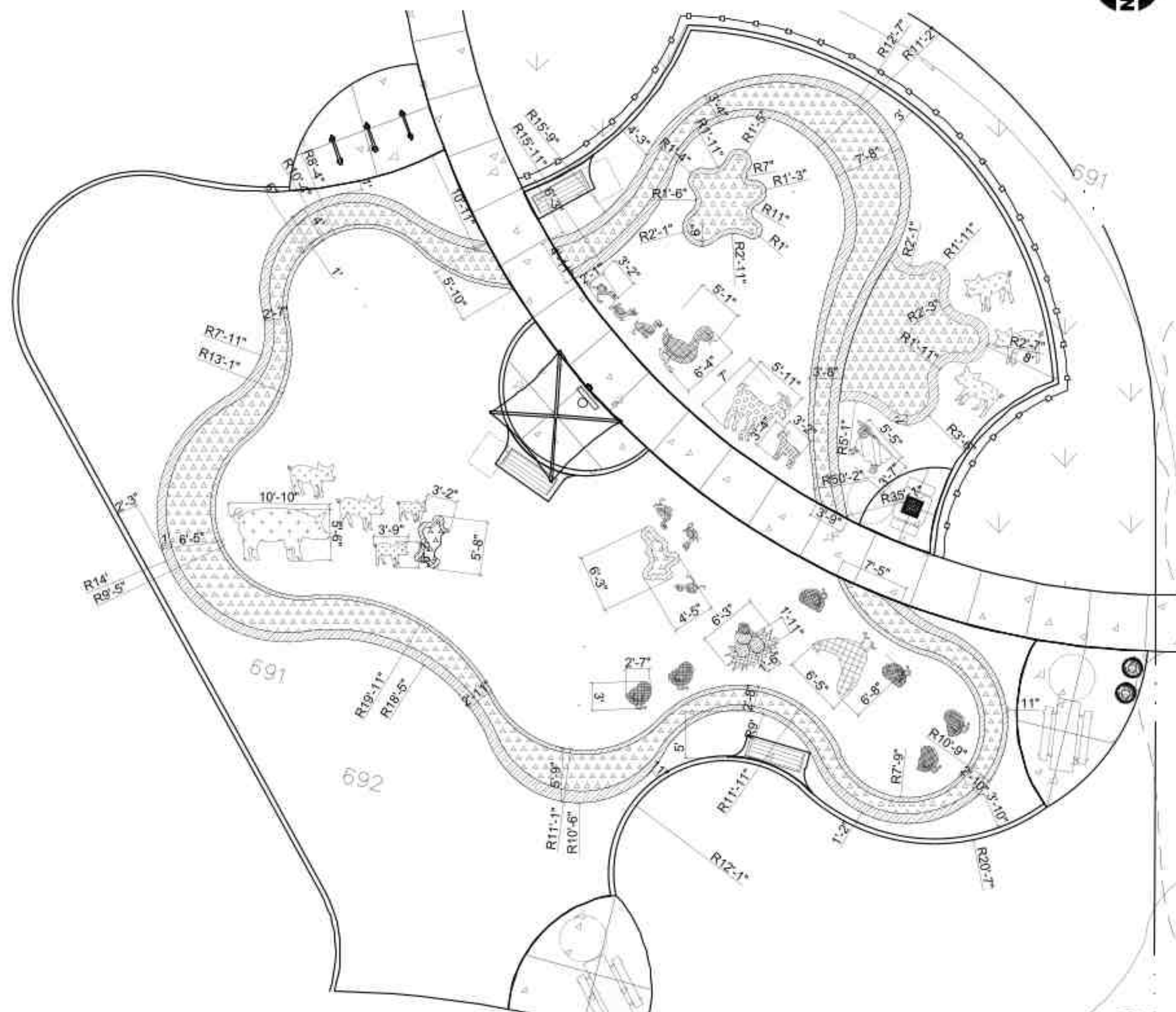
2 Poured-in-Place Surfacing Dimension Plan SCALE: 1" = 10'-0"
