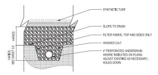
Underdrain in Turf Scale: 1"=1'-0"
